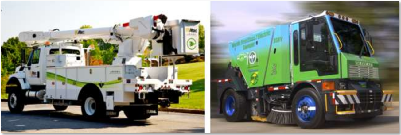
Figure 14. Bucket truck with Altec Industries JEMS system and Global Environmental Products electric sweeper.
