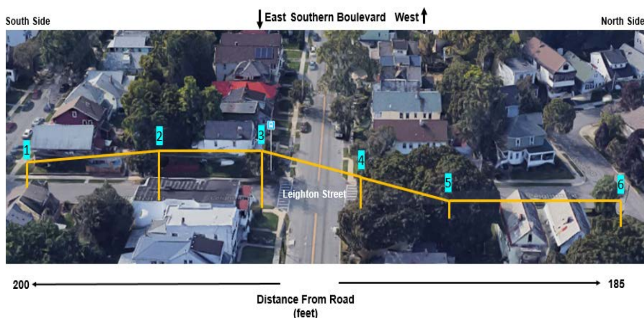
Figure 44. Portable Mini station Network Deployed across Leighton Street Perpendicular to Southern Boulevard
