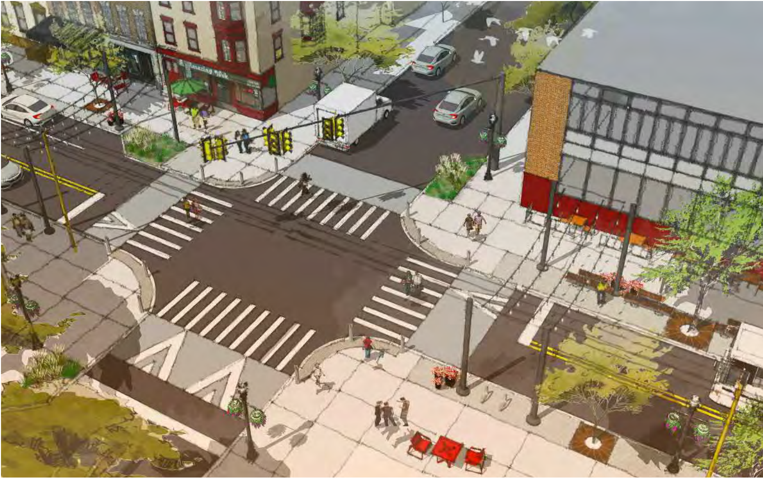
▲ Preferred Alternative. Raised intersection, curb extensions, decorative lighting, and green infrastructure shown at a typical minor signalized intersection.
