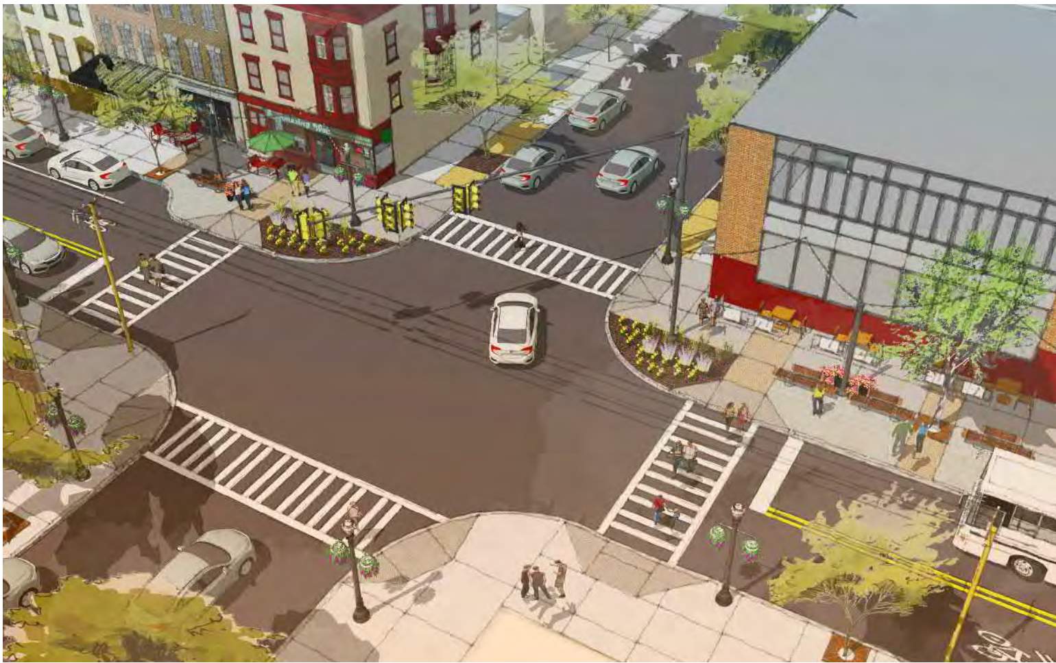
▲ Streetscape Design Alternative 1. Curb extensions and crosswalks shown at a typical minor signalized intersection.
