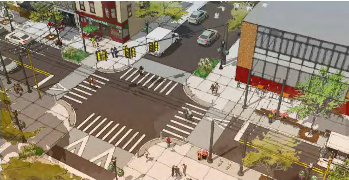
▲ Preferred Alternative. Raised intersections, curb extensions, decorative lighting, and green infrastructure shown at a typical minor signalized intersection.
