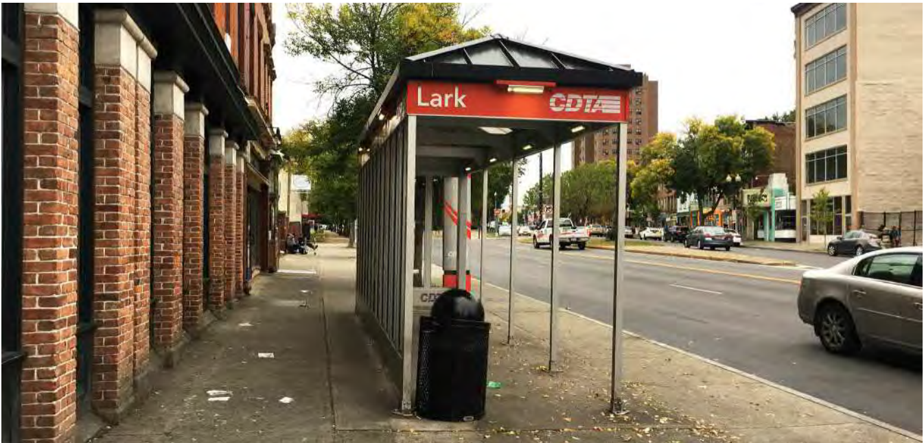
▲ The size and constrained sidewalk space associated with the bus shelter at the Washington/Lark bus stop on Washington Avenue creates a dark, uninviting corridor and obstructs pedestrian mobility. Proposed changes to address these issues include a 3 foot wide curb extension to create additional sidewalk space, a smaller bus shelter, and improved lighting.
