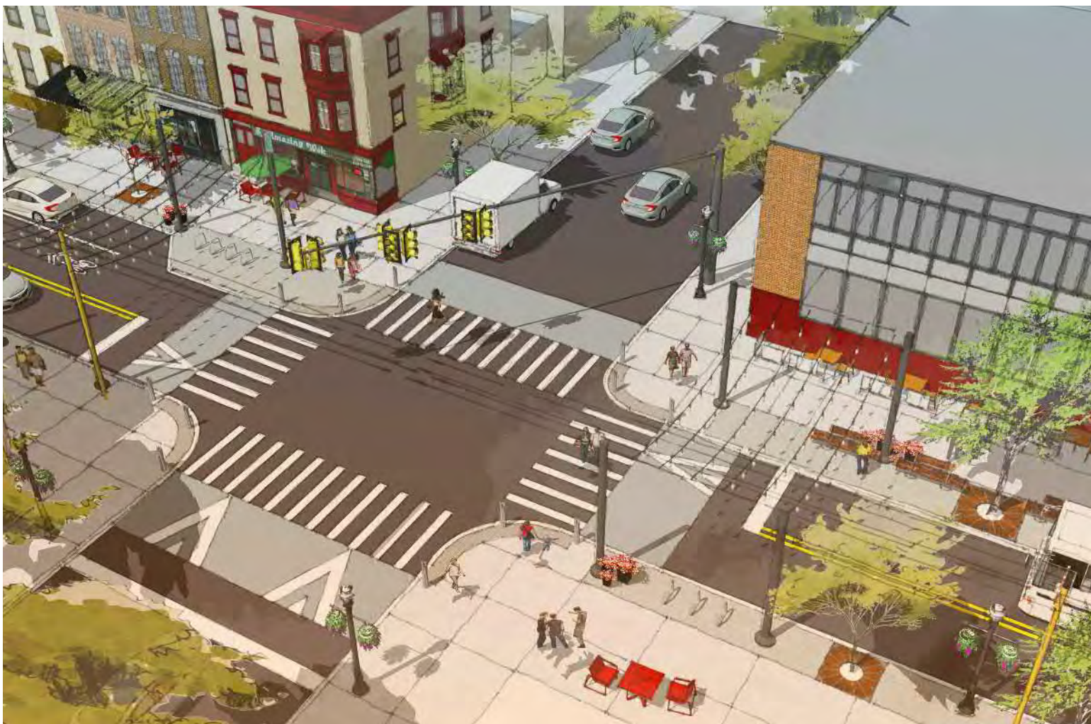
▲ Streetscape Design Alternative 2. Raised intersection and curb extensions shown at a typical minor signalized intersection.
