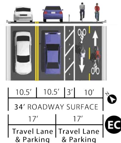
Figure 2-10: Cross-section of Church Street Cycle Track
